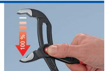
Press the button – open pliers completely
