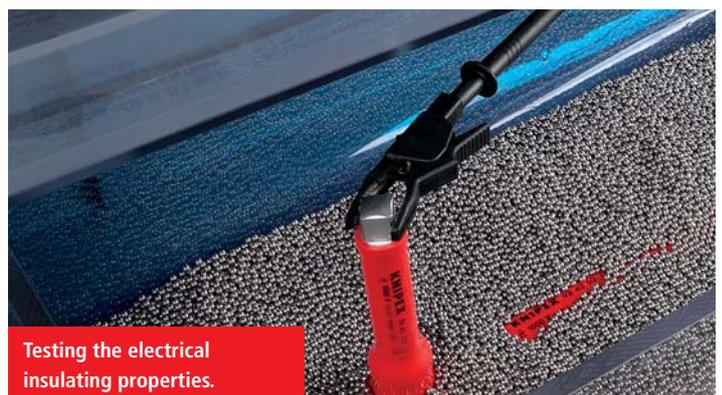
Testing the electrical insulating properties.
