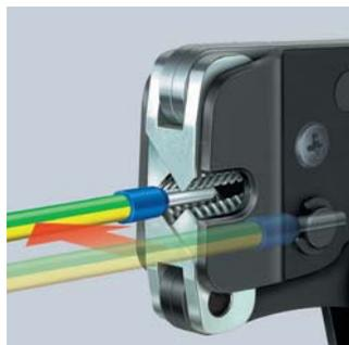
97 53 08: lateral loading of end sleeves (ferrules) up to 2.5 mm<sup>2</sup> parallelly from the side e.g. in confined areas
