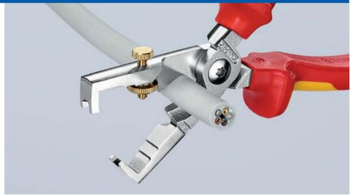
Induction hardened shear blade with precisely ground cutting edges for crushing-free cutting of copper cables of up to Ø 15 mm (5 x 2.5 mm<sup>2</sup>)
