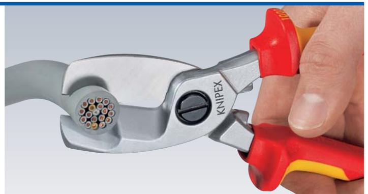
**Initial cut:** using the front cutting edge to cut the insulating sheath on larger cable diameters retains an ergonomic handle opening width.
