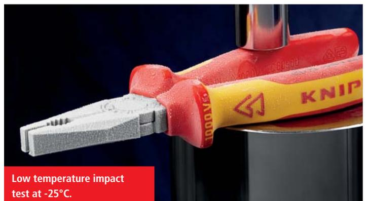
Low temperature impact test at -25°C.
