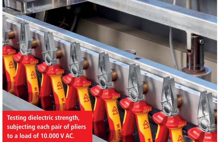
Testing dielectric strength, subjecting each pair of pliers to a load of 10.000 V AC.
