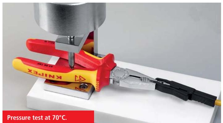
Pressure test at 70°C.
