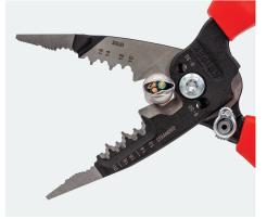
Shear type blades easily cut BX/MC cable
