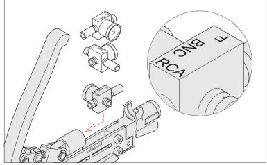
Inserting the connector insert in the correct position
