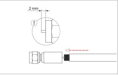
Connecting the coax cable with the compression connector
